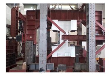
Fig. 2 Test set-up for coupling beam
