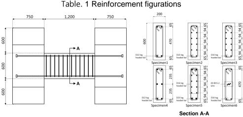
Fig. 1 Test beam geometries
